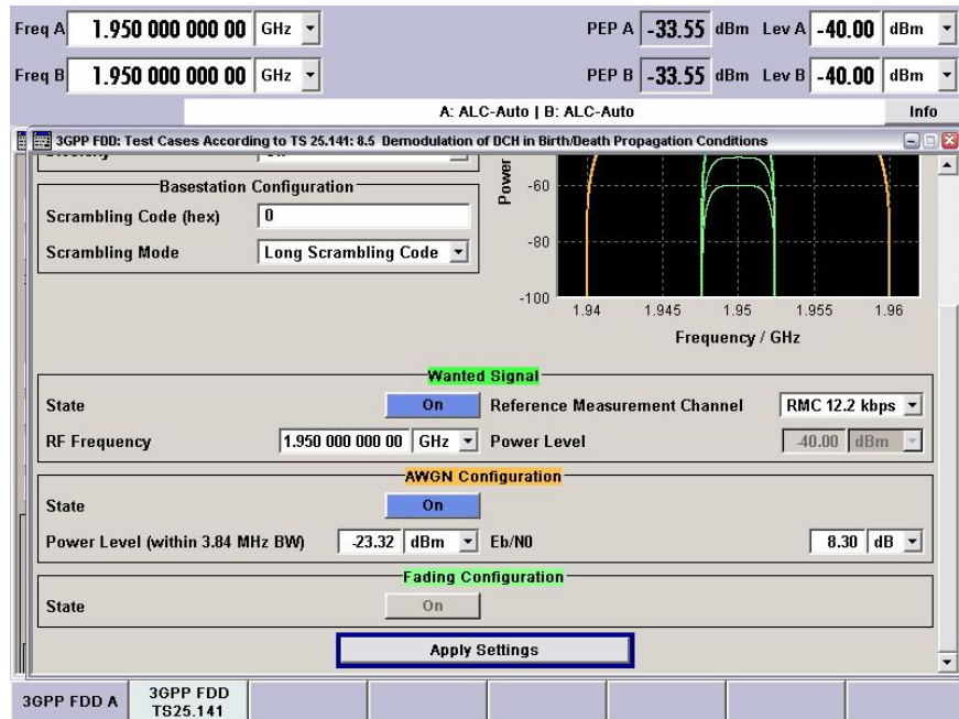
Figure 8.2.1_2: How to switch off the AWGN on SMU Test Wizard.
